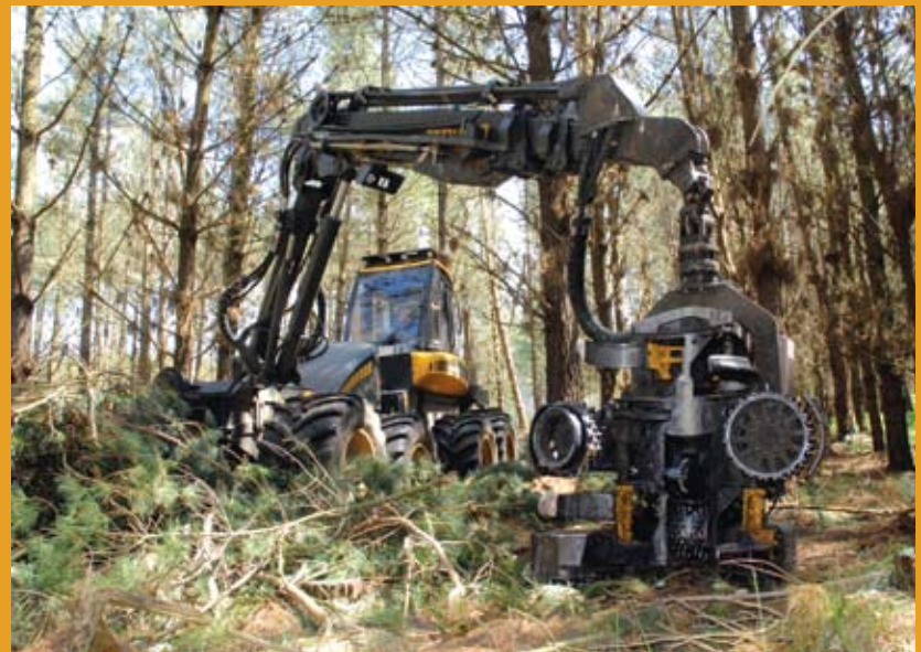
The Ponsse Ergo harvester and the H7 (70cm) head is powerful. "The feeding force is phenomenal. In this small, rough, branchy pine, I am cutting 15 to 20 metres an hour. In clean timber, you can get up to 60 to 70 metres an hour."
