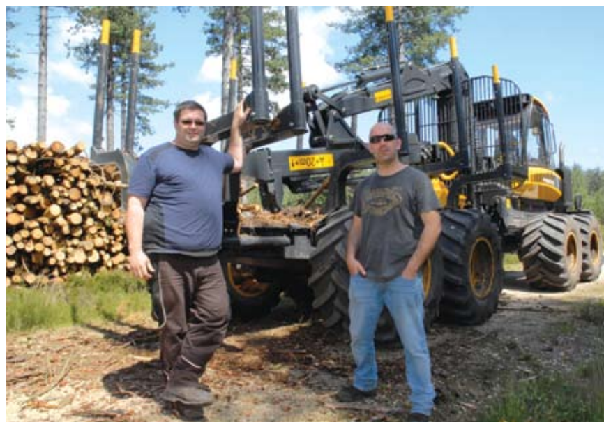
Forwarder driver Philip Palmer (left), who has worked with Nick for the last 2½ years (since Rod retired), and Nick Cooper of Cooper Forestry, beside the 14-tonne capacity trailer of Cooper Forestry's new forwarder, the 275hp Ponsse Buffalo.
