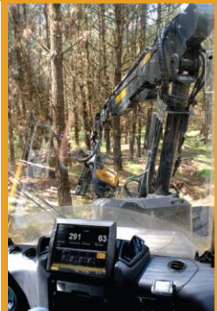
Inside the cab of Nick's Ergo harvester, with the Opti 5 system on the computer screen, showing length, diameter and optimisation.
